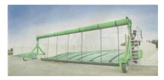
Retractable bunker cover system uses a set of A-frame gantries that run outsidé bunker walls, quickly unrolling or rolling up a weatherproof cover over silage. It's held in place by filling overlying hoses with water.
